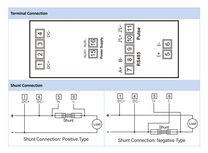
\*\*Remarks: If the customer needs to add a circuit breaker, it cannot be added between the signal lines of the DC- and shunt lines.
